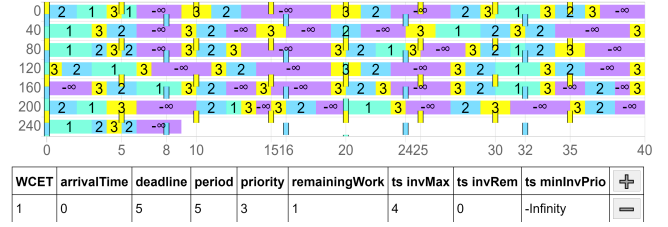
Figure 2: Screenshot of the interactive simulation TaskShuffler in Action ( https://www.simonlanger.com/uni/KvBK/?render=3 ): Each row in this diagram represents one hyperperiod (i.e. the smallest common multiple of all tasks' periods, here: 40); time is arranged in row-major order. With FP-scheduling, every row of this diagram would be exactly the same; TaskShuffler's randomization, though, manages to significantly reduce the predictability of task executions. Tasks are labeled with their respective priorities – from highest to lowest: 3 > 2 > 1 > -\infty (idle task). Note that two consecutive executions of the same task are displayed as one contiguous horizontal segment. At the point in time this snapshot was taken, the remaining inversion budget of the highest priority task is 0 ( ts invRem ) while it has remaining work, so it will definitely execute in the next time slot; this ensures that the task does not miss its deadline (depicted by the vertical dashed yellow line in column 10) – once the job is completed and task 3's next job released, the remaining inversion budget will be reset back to task 3's maximum inversion budget ts invMax = 4.
